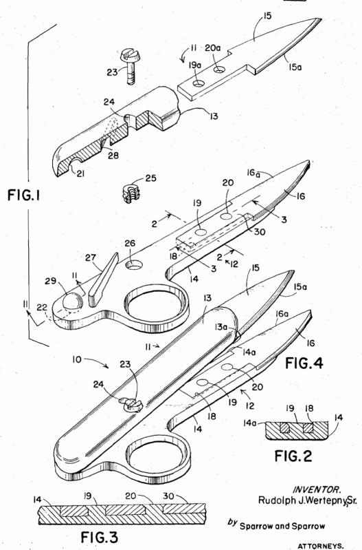
BLADE-TYPE CUTTING IMPLEMENTS AND METHOD OF MANUFACTURE
