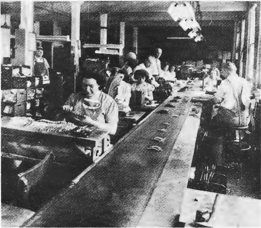
Assembling scissors at Wiss. This photograph of the inspection and rework department of Wiss, in 1948, was part of a group of photographs taken in honor of Wiss' 100th anniversary.
