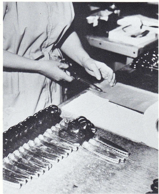
—Final inspection: shears undergo rigid cutting tests and examination before packaging.
