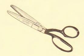
The primary importance of pinking shears is the finishing of inside of seams of dresses and other garments to make them ravel-proof. Pinking shears eliminate tedious hand pinking, overcasting, picoting, and bias binding.
