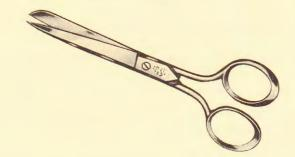
Generally these scissors have one rounded and one pointed blade. They vary in length from three to six inches.
