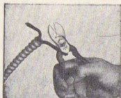
Crushing rubber insulation before cutting.
