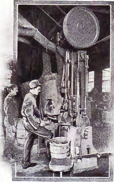
Welding the hard cutting edge to the tough frame
