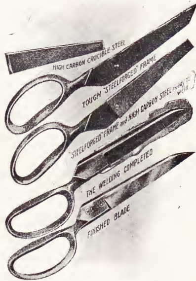
Showing WISS Shear Blades in various stages of development.
