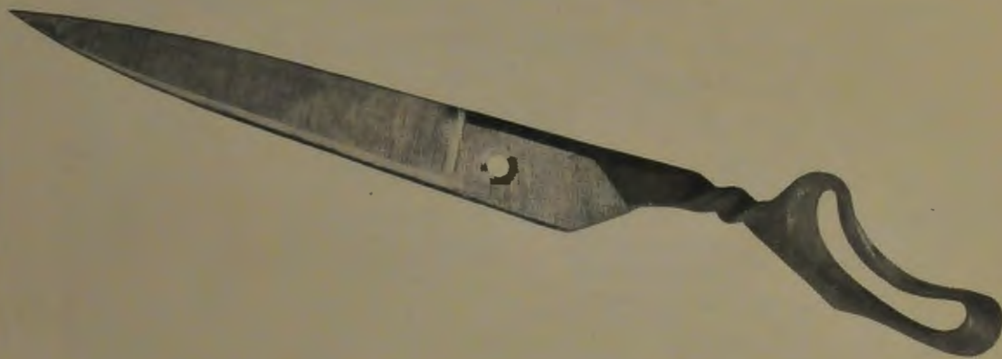
Showing how it is possible to twist and bend the handles of Wiss Shears without breaking them
